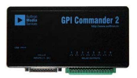
The Application GPI Commander is a free application that can be downloaded from our website www.softron.tv. GPI Commander can control one or more GPI Commander 2 boxes via USB. These boxes have 8 outputs and 24 inputs.
