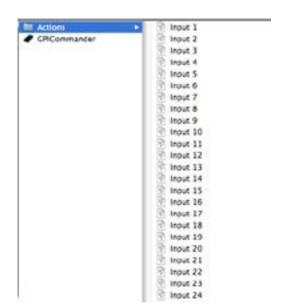
The AppleScript named "Input 1" will be triggered when the state of the Input 1 will change. The AppleScript named "Input 2" will be triggered when the state of the Inputs 2 will change, etc...
