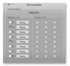
Each GPI Commander Box has a unique serial number that is shown in the "Serial Number" area on the top of the User Interface.
